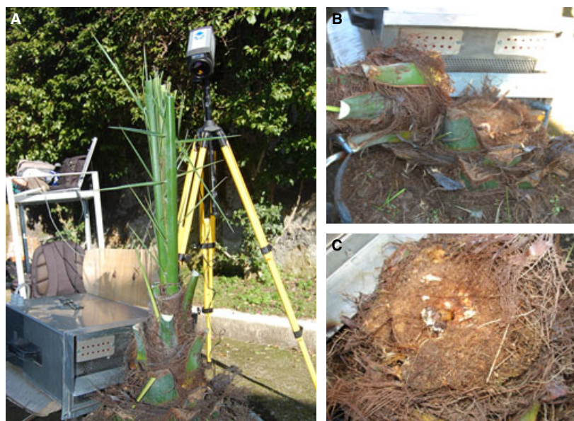
Fig. 4 Microwave treatment of palm: (A) experimental setup; (B) preliminary cut of the palm; (C) section of the palm with larva inside.
