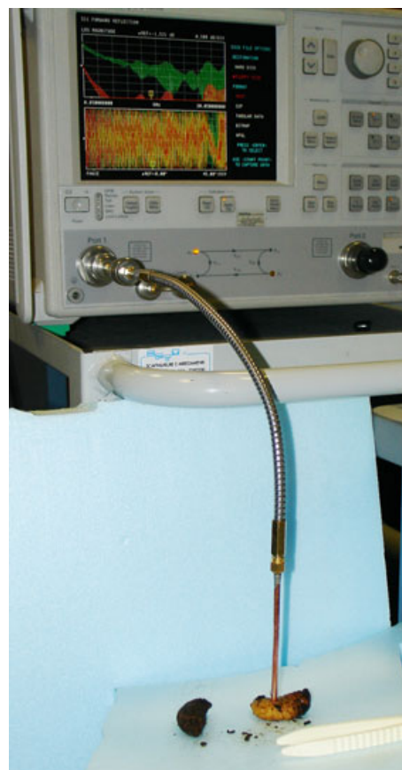
Fig. 1 Experimental set-up for permittivity measurements with the open ended coaxial cable technique.
