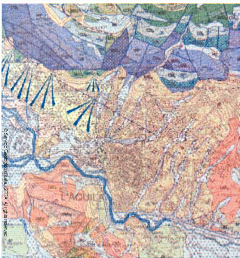
Geological map of L'Aquila (1:50,000 sheet 359) published before the 2009 earthquake showing lighter tones indicative of softer ground and widening blue lines to indicate debris flows of unconsolidated material
